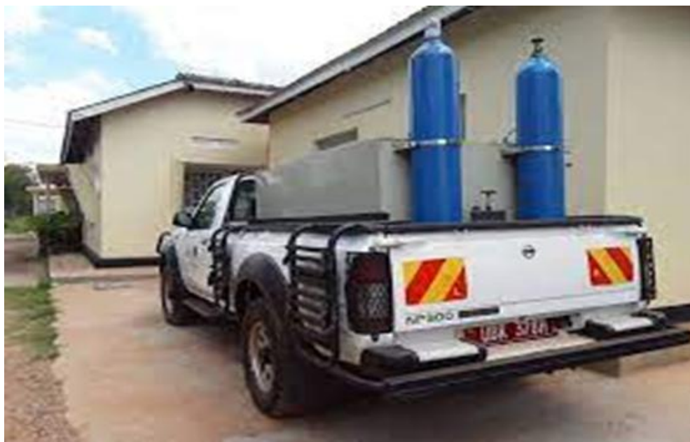
Figure 16 Live fish transporting tank with Oxygen cylinders mounted on a pick-up (NaFIRRI, Uganda)
