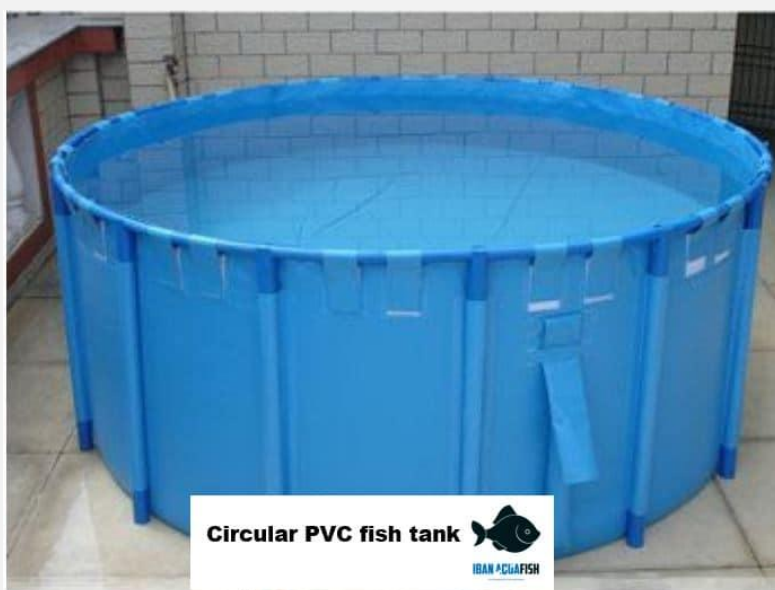
Figure 13 Circular PVC fish tank set up (Source: IBAN Aquafish Solutions and Consultancy Limited)
